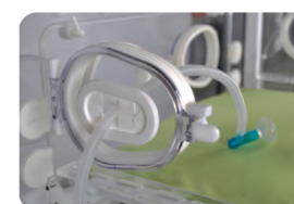
Grommets and port holes
