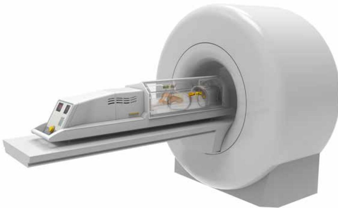
MR Diagnostics Incubator System **nomag®IC ADVANCED** in MRI
